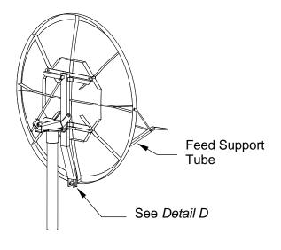
A). Connect the feed rods to the feed support tube with (items: 4, 6, 7) and with [2] of (item 5).
